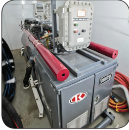
Enviro Vacuum Shack Ketek's Vac Shack is used in cold weather applications to provide shelter for the Enviro-vac and prevent freezing problems.
